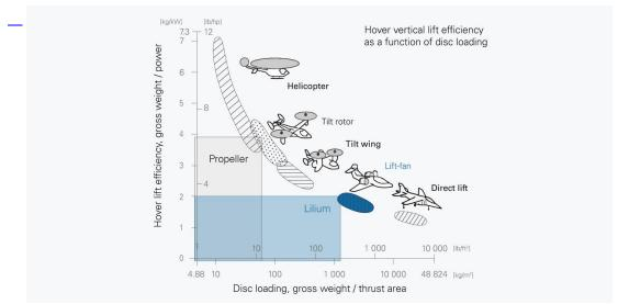
Lilium will lose a significant amount of efficiency in the hover phase due to its small rotors and high disc loading Lilium
